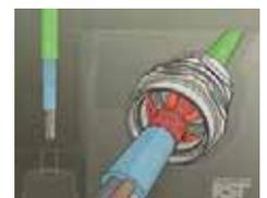
Using the contact system within the Euro-Top screw connection, the conducted cable can be contacted not just at the end of the cable, but also when the cable is fed further into the housing. As illustrated below, this only requires a short piece of the cable sheath to be removed within the screw connection.
